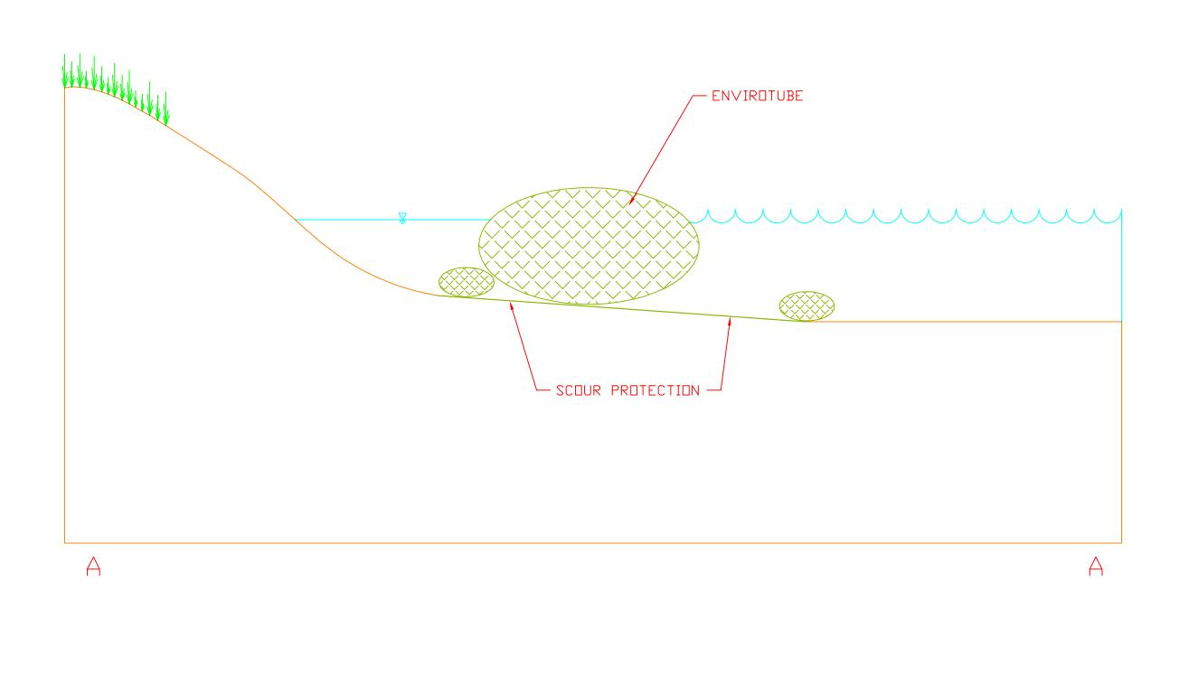
EMERGENT OFFSHORE BREAKWATER DETAIL A
